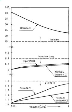
When normally closed: MS-136 single item condition When normally open: MS-136 and MS-136-C (P) coupled condition
