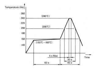
When hand soldering is used, use a tip temperature of 280°C or less and a soldering time of 3 seconds or less.
