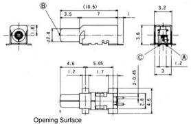
The circuit structure is as described below. Between (A) and (C): Normally closed Between (B) and (C): Normally open
